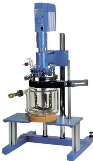
The IKA® LR-2.ST system is a modularly designed miniplant reactor system, planned and designed to simulate and optimize chemical reaction processes as well as mixing, dispersion and homogenization processes at a model scale with a maximum volume of 2000 ml.
