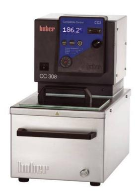
Heating Circulator Bath with housing, bath and all moistened parts are made of stainless steel. With cooling coil for water-cooling, pressure- and suction pump made of industrial plastic material. With adjustable overtemperature protection according to DIN 12876. CC3: Automation capable
